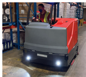
Safe Eyes forward operator design, standard LED front and rear lights
