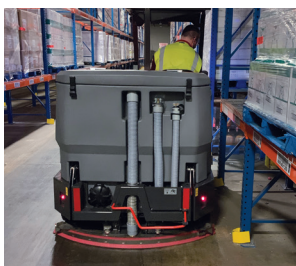
Productive Clean a 9ft aisle in 2 passes (55" with side scrubbing brush)
