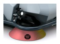
Dust-free cleaning: The optional pre-sweep/vacuum unit can be equipped with Dust Stop – our disc brush jacket providing dust-free sweeping & vacuuming.
