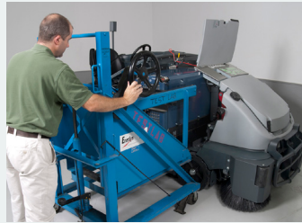
Install fuel cell into CS7010
