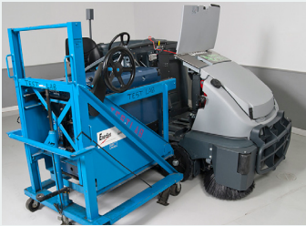
Lift the fuel cell to the height of the machine
